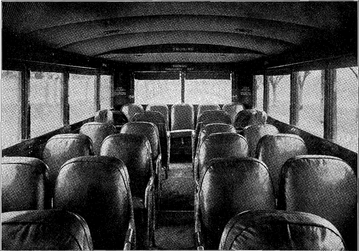
INTERIOR VIEW OF "FAGEOL" 27-PASSENGER SEDAN MOTOR COACH, SHOWING SEATING ARRANGEMENTS, ETC.
